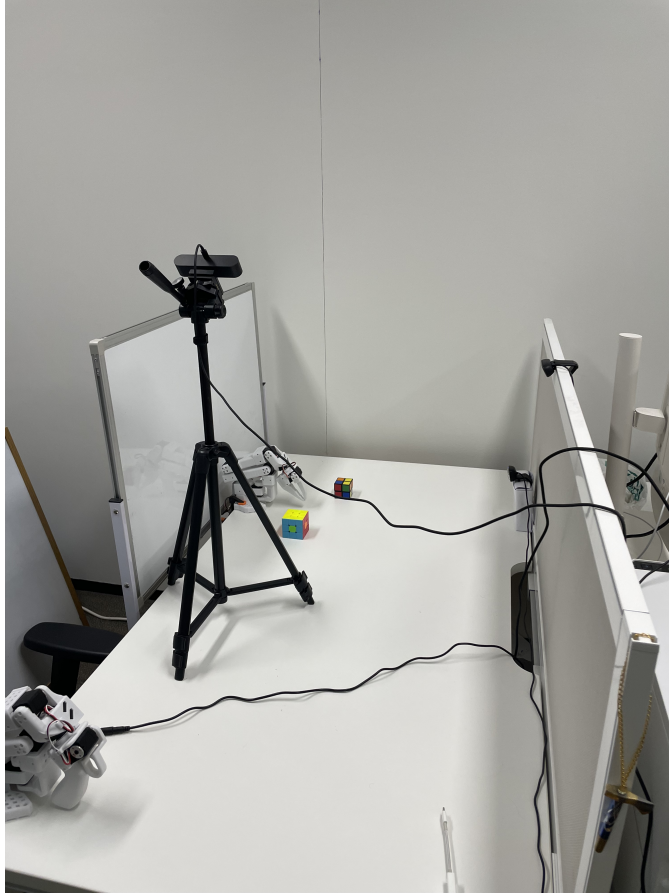
Figure 8. Experimental tabletop manipulation setup with a Lenovo top camera mounted on a tripod providing an overhead view of the white workspace, a front-facing Microsoft LifeCam attached to the desk divider, and a Logitech auxiliary camera used for task monitoring, reward computation, and partitioning the workspace into discrete zones to curate balanced and diverse training data. A 3D printed SO-101 robotic arm and gripper operate on a colored training cube and a Rubik’s cube on the central table, with whiteboards, an office chair, and USB cables routing connectivity between cameras and the control machine.
