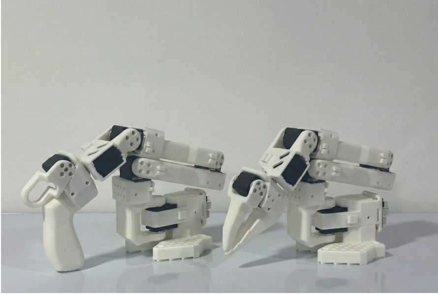
Figure 7. A pair of white 3D-printed SO-101 robotic arms with black ST-3215-C0xx servos, resting side-by-side on a clean white surface.
